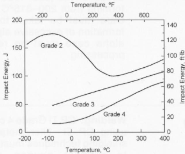
Elevated Temperature Mechanical Properties for CP Ti Grade 4
